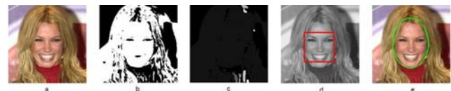
Fig. 5. Example of face detected by the luminance branch and validated by the chrominance channel (but it is not detected by the chrominance channel!): (a) original image; (b) skin color segmented image; (c) connected components; (d) luminance detection result; (e) best-fit ellipse.
