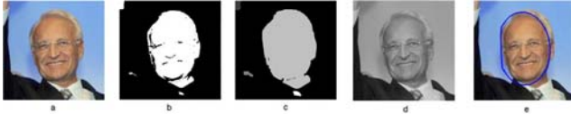
Fig. 6. Example of face detected by the chrominance branch and validated by the luminance channel (but it is not detected by the luminance channel!): (a) original image; (b) skin color segmented image; (c) connected components; (d) luminance detection result (failure of detection); (e) best-fit ellipse.
