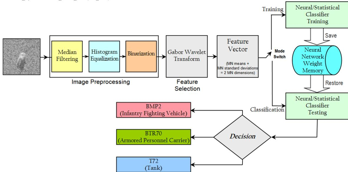
Fig. 1. Flowchart of the ATR cascade.
