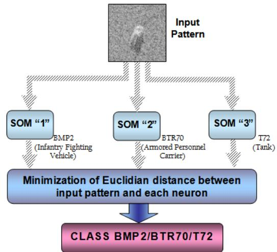
Fig. 4. The classification phase of the CSOM model.
